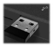
To connect an OTG device, gently insert it into the <u>Type-A connector</u> next to the microSD card reader slot. It will only fit in correctly when the side with the 2 openings is facing you (per the illustration).
