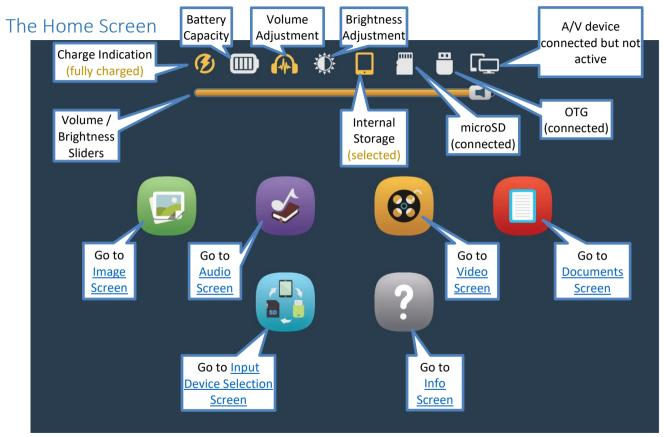
Above: Envision is connected for charging (completed), an external audio device is connected, A/V device is connected (but not active), the volume is being adjusted, external microSD and OTG are connected but Internal Storage is the selected input.
