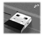
To connect an OTG device, gently insert it into the <u>Type-A connector</u> next to the microSD card reader slot. It will only fit in correctly when the side with the 2 openings is facing you (per the illustration).
