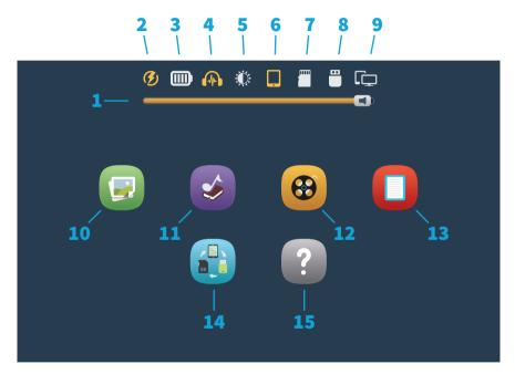
Image Above: Envision C01 is connected for charging (completed) (2), battery is full (3), an external audio device is connected (4), A/V device is connected (but not active) (9), the volume is being adjusted (1+4), and external microSD and OTG are connected (7+8) but Internal Storage is the selected input (6).
