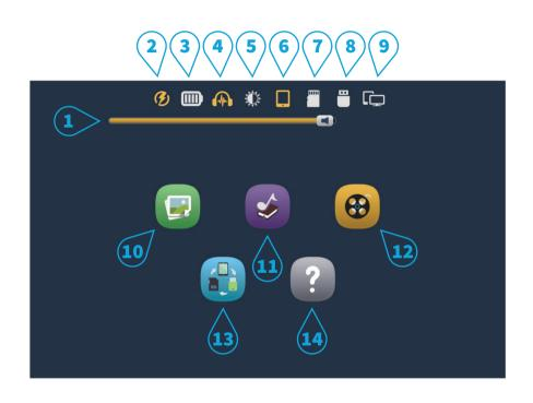
Image Above: Envision B02 is connected for charging (completed) (2), battery is full (3), an external audio device is connected (4), A/V device is connected (but not active) (9), the volume is being adjusted (1+4), and external microSD and OTG are connected (7+8) but Internal Storage is the selected input (6).
